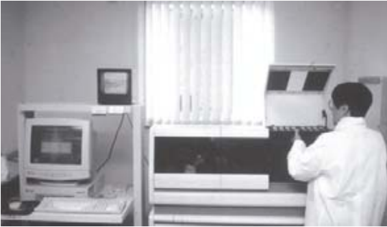
Fig. 9 The trays of Pap smears are loaded into the FocalPoint® instrument. It takes approximately 8 minutes to scan one slide.
