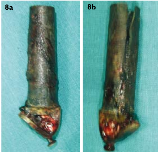
Fig. 8 Photographs show the removed rear end of the gun barrel. Note the breach in the tube and in the rear end.
