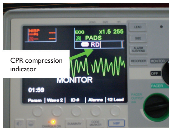
Fig. 2 Defibrillator screen display incorporating QCPR feedback indicators (Zoll E series). When complete filling of the CPR compression indicator has not been achieved due to diminished compression rate or depth, the E Series will display the letter R for rate and/or the letter D for depth to assist the rescuer in determining whether chest compression rate or depth should be increased. When appropriate rate and depth have been achieved, these letters will disappear from the display field. A voice prompt option is also available.
